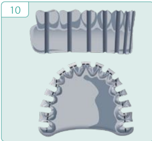
Cut a 2.0mm wide groove in center of each tooth joining the lines representing the middle of each tooth and greatest concavity of the tissue side.
